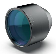
The new Futonics product line of F-Theta lenses is based on crystal lenses made of zinc selenide and calcium fluoride. Effective focal lengths of 170 mm and 345 mm are available.
